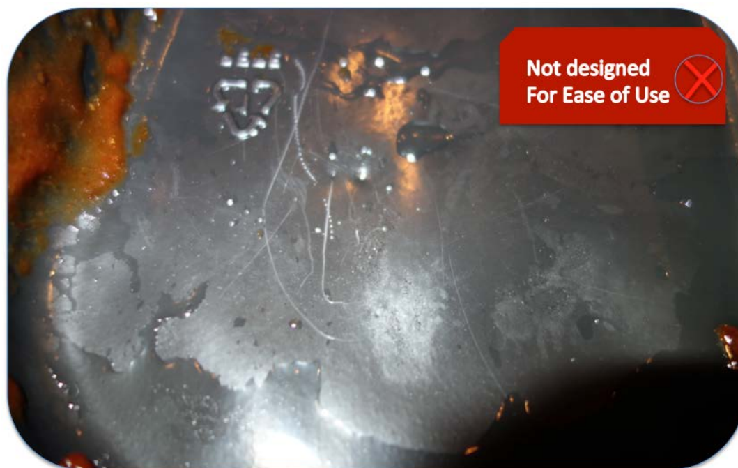
Figure 14: Example of a plate scraped and punctured by a fork.
