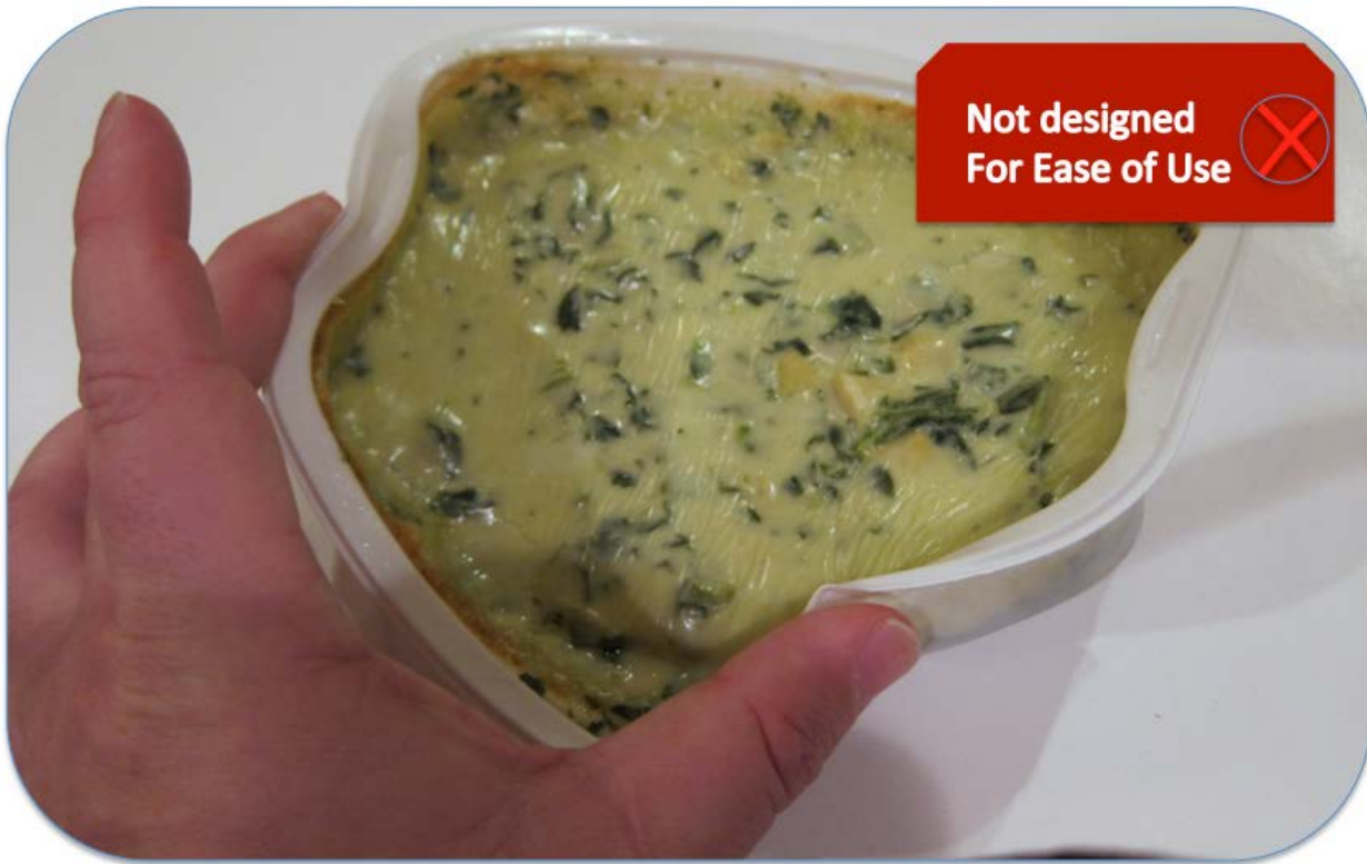
Figure 13: Image of plate losing rigidity after heating.
