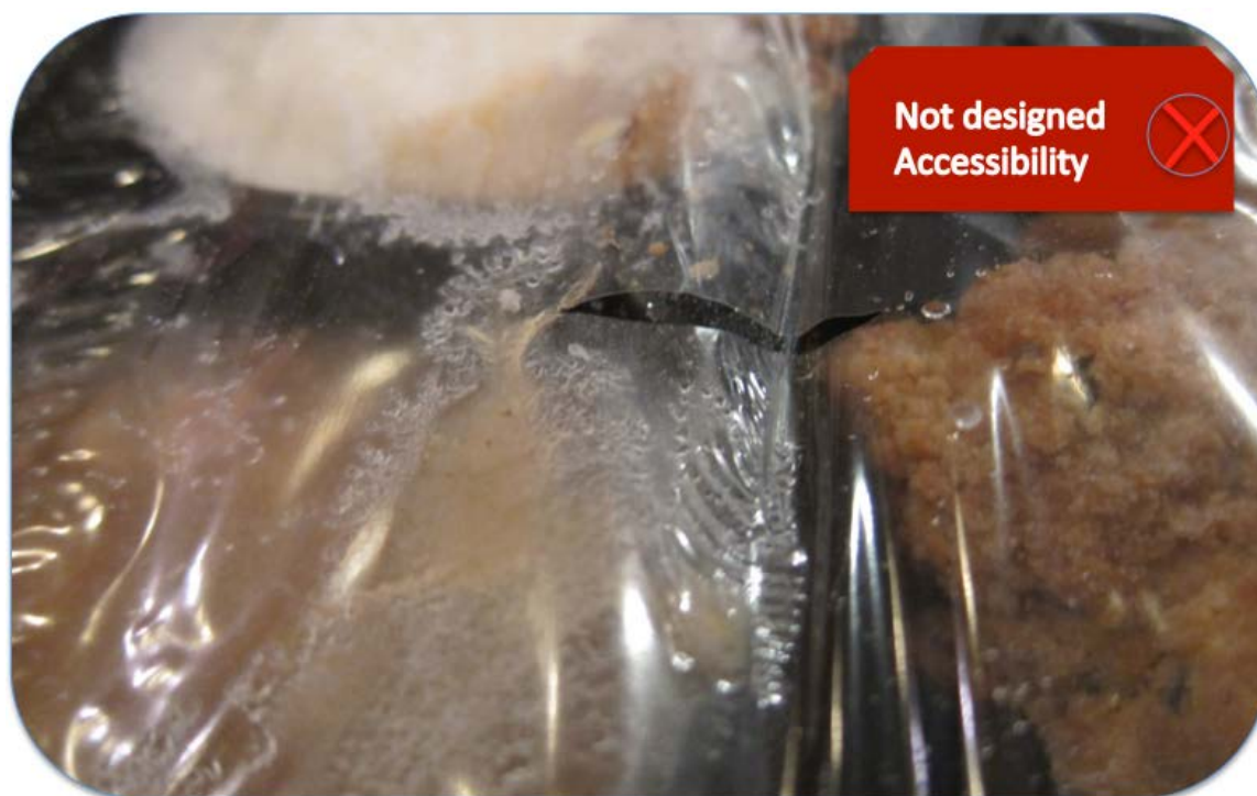
Figure 2: Film membrane ruptured during transport.
