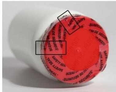
Figure 25: Perforations (outlined in black boxes) in the safety seal are not visible
