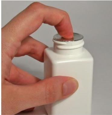
**Figure 16: Seal can be punctured with a fingertip**
