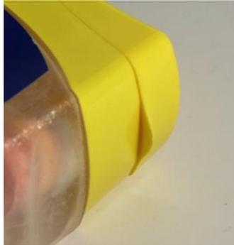
**Figure 9: Sharp lift tab**
