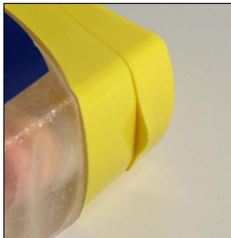
**Figure 9: Sharp lift tab.**
