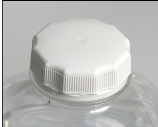
**Figure 8: Cap with sharp edges.**
