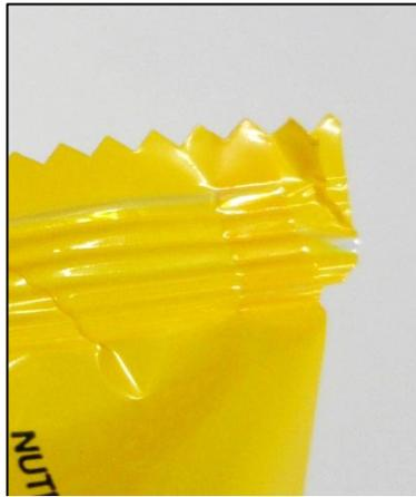
Figure 13: A serrated edge.
